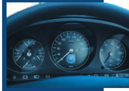
△ Dial set with dual temp gauges and OLED display.
